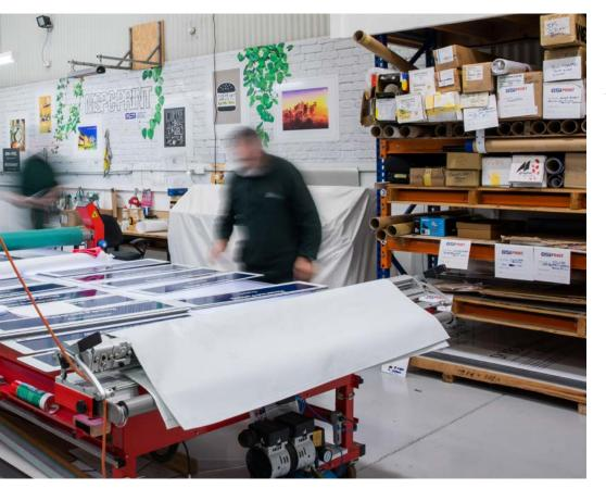
workflow. Equipment includes HP Latex R1000 hybrid flatbed / roll-to-roll printer, a Canon Arizona flatbed, a Mimaki roll-to-roll, with an Epson F2260 direct-to-film printer and a heat press, a Roland DG Versacamm UV for promotional products, which has seen the best part of 20 summers, and a Zund cutting table. Varnakulasingham says, "We have the means to handle a wide range of work, producing high quality jobs. Our customer base is loval."
